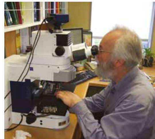
Figure 4. Ian Raine, GNS Pollen Lab, using a compound microscope designed to show pollen grains on the computer screen and in the microscope as well as take high resolution photographs.
