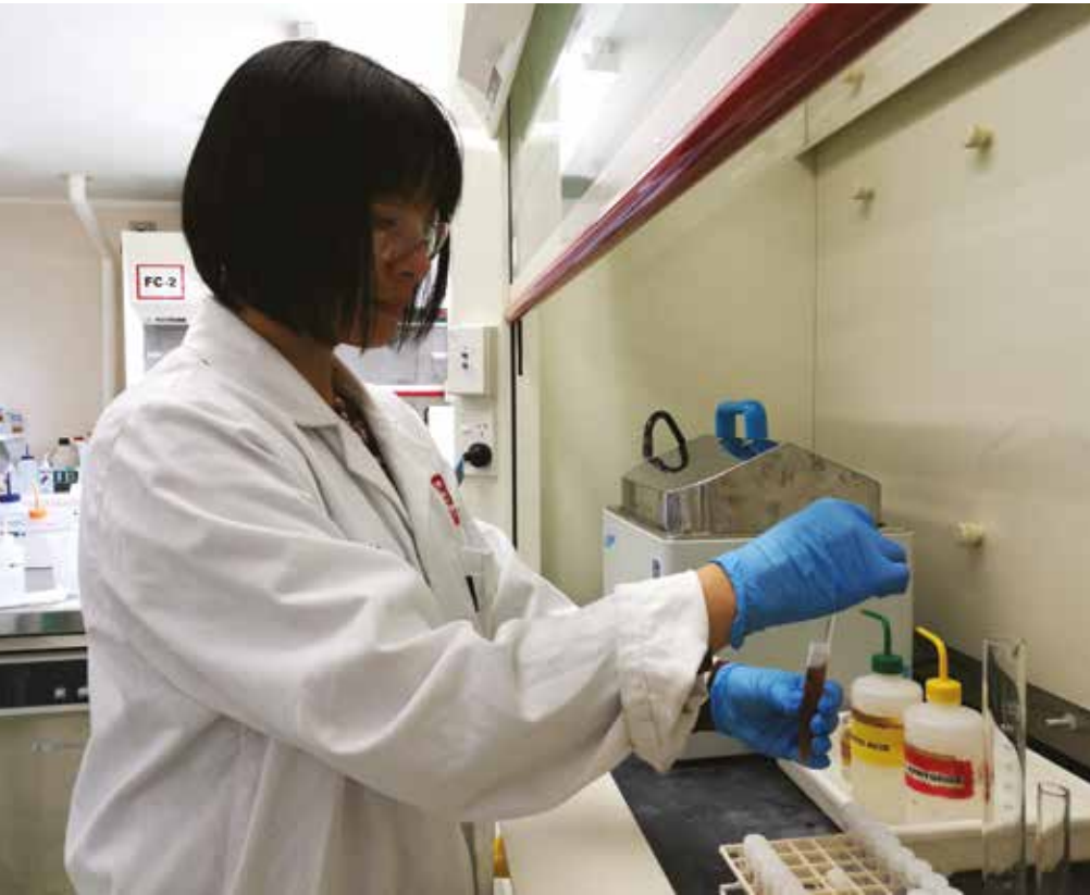
Figure 3. Xun Li, GNS Pollen Lab, processing pollen by the acetolysis method which requires a chemical fume hood that handles the acid fumes.
